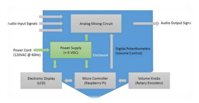
We chose a Raspberry Pi as the main controller for the digital circuitry. For volume knobs we chose Rotary Encoders (Position is not stored, Clockwise and Counterclockwise rotation is recorded digitally.) A PCB containing our power supply and analog mixing circuit is housed in our enclosure. The analog mixing is done with digitally controlled potentiometers so that the volume can be adjusted digitally from the Raspberry Pi. An electronic display is also controlled by the Raspberry Pi.
